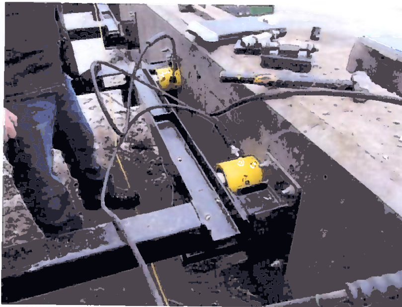
Photo 18: 50 ton capacity hydraulic rams (x2) used to introduce buttressing load into precast pre-stressed exterior wall panels
